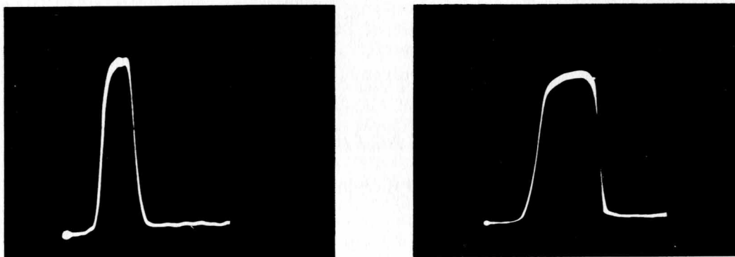
Figure 2. (A) 0.01 \mu sec Pulse Through \text{hp} 460BR Amplifier (B) 0.02 \mu sec Pulse Through 3 Amplifiers in Cascade
